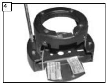
Remove the 4 screws attaching the Mounting neck the mounting plate. Retain the 4 screws for re-assembly.
